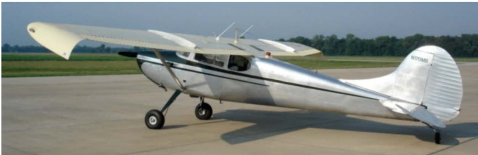
Figure A-8 Drooping the Wing Tips
